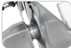
More space between blade and body machine
