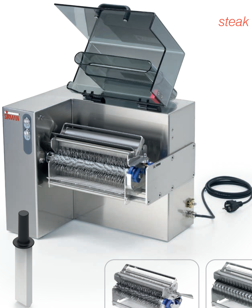
da 10 mm con 48 lame da 15 mm con 32 lame Cutting blade assembly: 10 mm with 48 blades 15 mm with 32 blades
